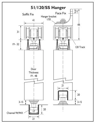
For MDF doors 19-23mm you must use hanger 52/120/SS and for doors 24-48 there is an option of surface mounted or routed (51/120/SS or 57/120/SS)
